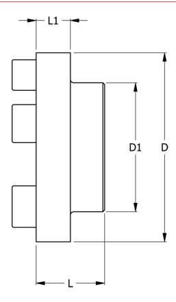
D = 125 D1 = 100 L = 50 L1 = 18 Max bore = 55 Torque (N m) = 240
